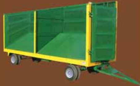
ÇİFT DİNGİLLİ, 8 TEKERLEKLİ, SOLA DEVİRMELİ PAMUK RÖMORKU SIDE TIPPING TRAILERS OF COTTON, DOUBLE AXLE, EIGHT WHEELS
